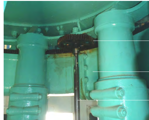
Vertical shaft continuous with shaft in photo above. Driven through bevel wheels by a horizontal main drive Main drive Bevel wheel on main shaft Foot Winding shaft Squared for turning by a manual crank Maker's insigne
