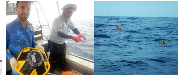
Figure 1. Left: Adrien Moineau and William Sokimi connect the wave buoy to the FAD; Right: the low-profile wave buoy is attached to the FAD and starts sending data. (Images: SPC)
