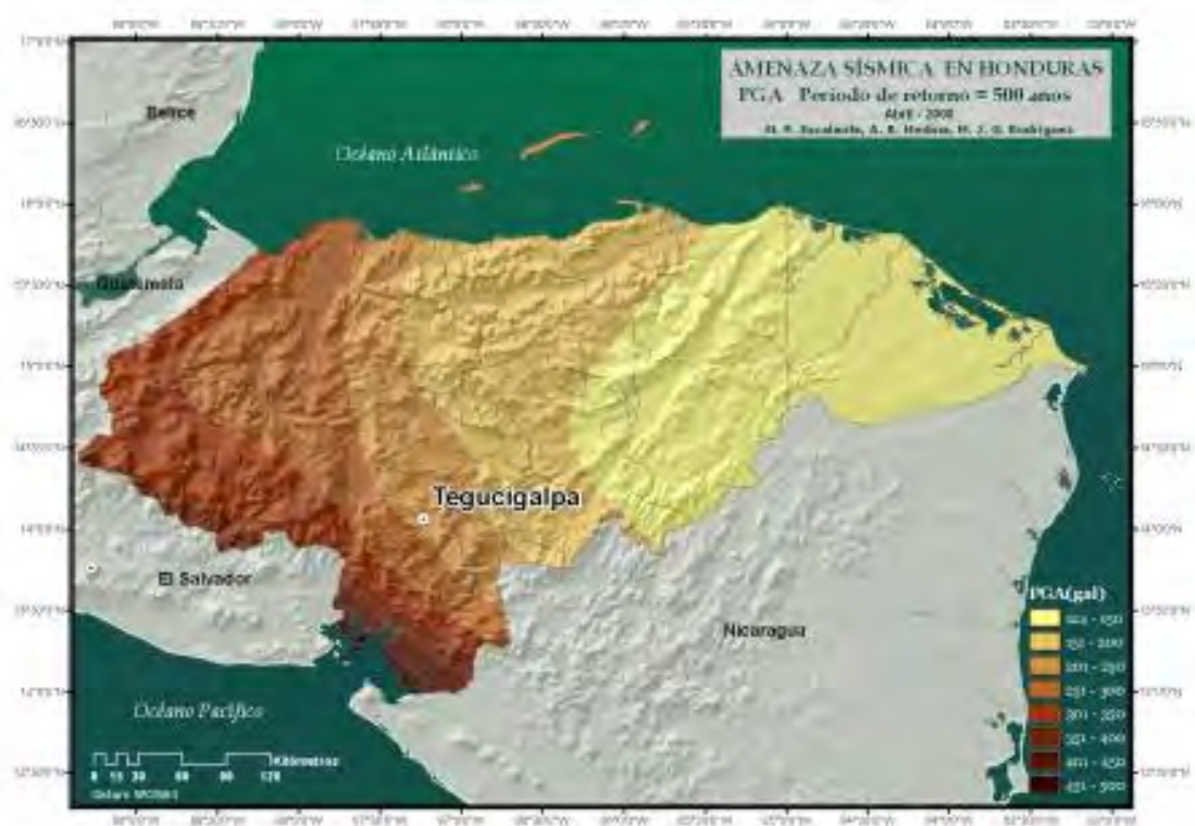
Figure 2.6.6 Seismic Hazard of Honduras by RESIS II (PGA, Return Period 500 years) (Source: RESIS II Report)
