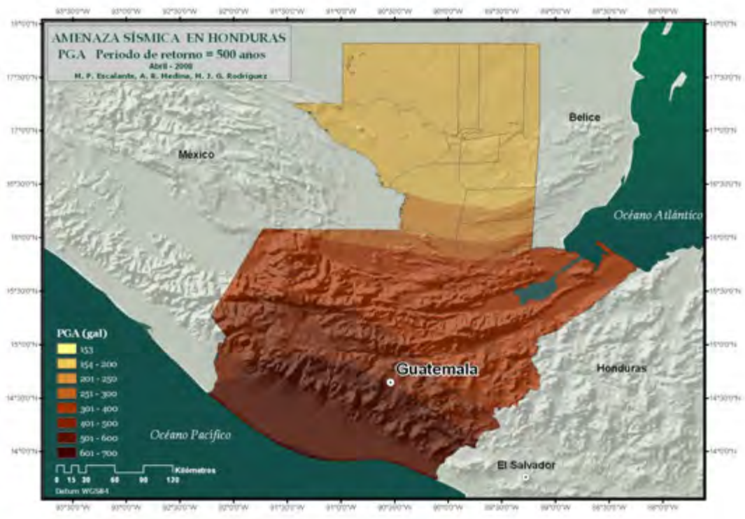
Figure 2.3.10 Seismic Hazard of Guatemala by RESIS II (PGA, Return Period 500years) (Source:RESIS II Report)
