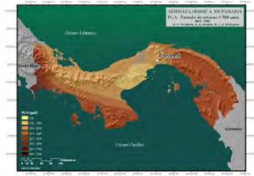
Figure 2.5.9 Seismic Hazard of Panama by RESIS II (PGA, Return Period 500 years) (Source: RESIS II Report)
