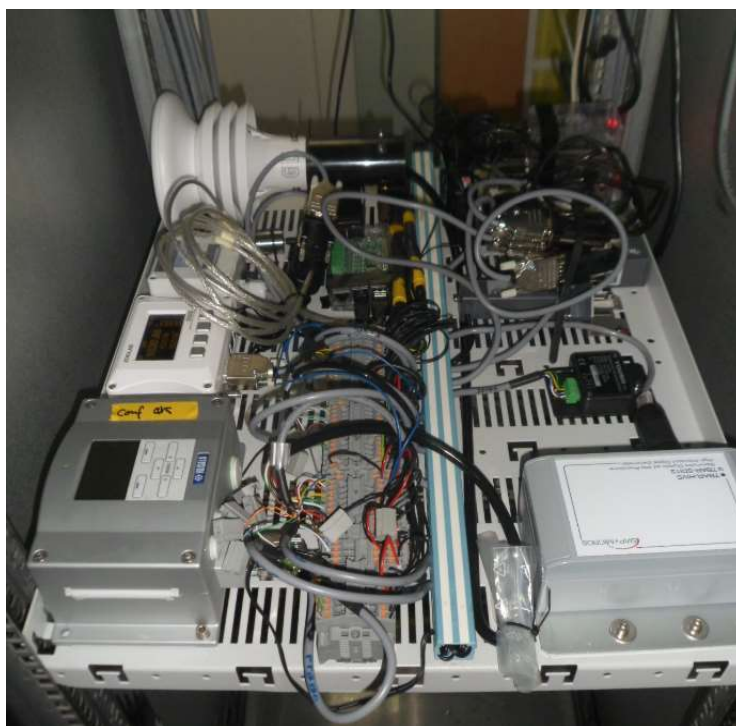
Figure 15- Integration of 13 barometers on Research Vessel L'Atalante
