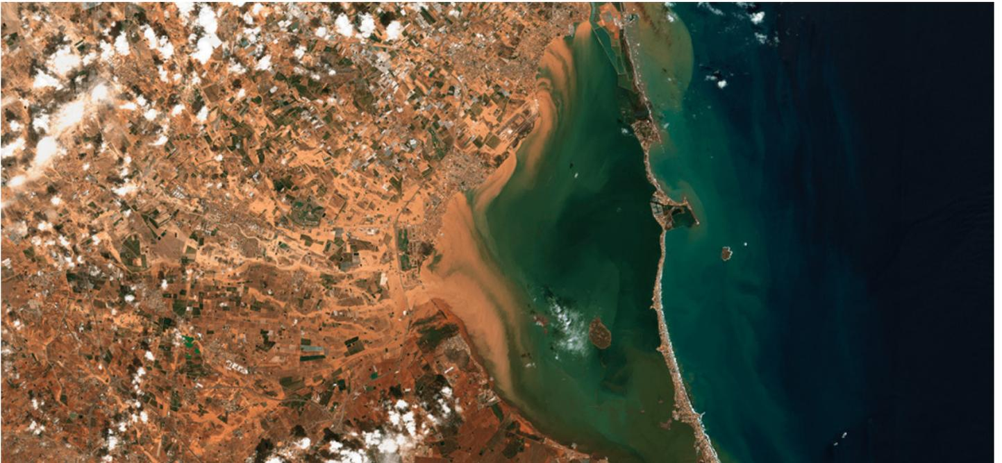
Fig. 3. Satellite image (Sentinel 2) after torrential rainfall in September 12<sup>th</sup> and 13<sup>th</sup> in the Mar Menor watershed. Tons of terrigenous sediments, carbon, nitrogen and phosphorous are dragged by water runoff from agricultural lands into the Mar Menor lagoon (downloaded from <https://www.copernicus.eu/>)
