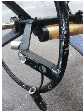
6200025 buoy: Wind sensor bracket broken.
