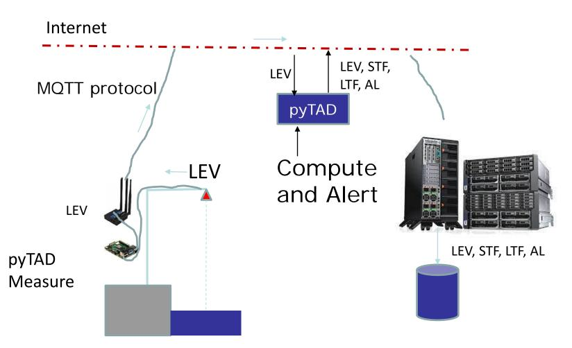
IDSL measures only Computing and alerting demanded to an external programme, running in a computing center
