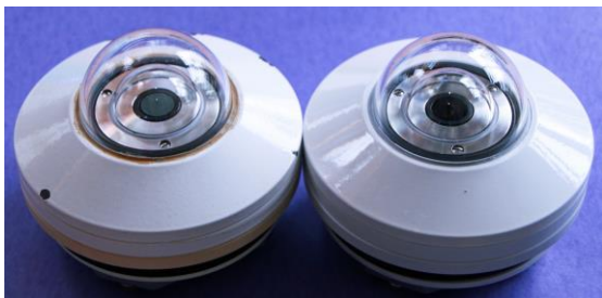
Degradation of optical black paint on incoming shortwave radiation sensor
