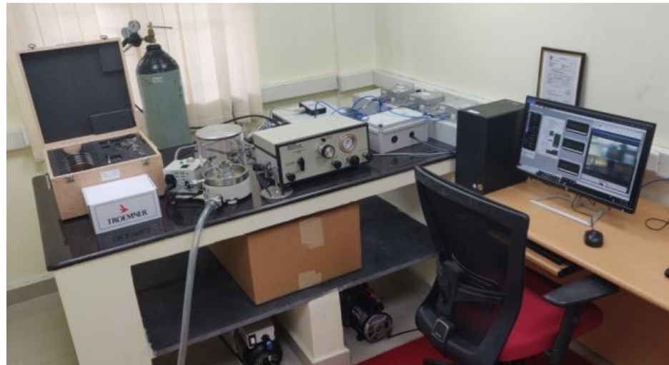
Digital Gas Piston Gauge- Barometric pressure sensor calibration
