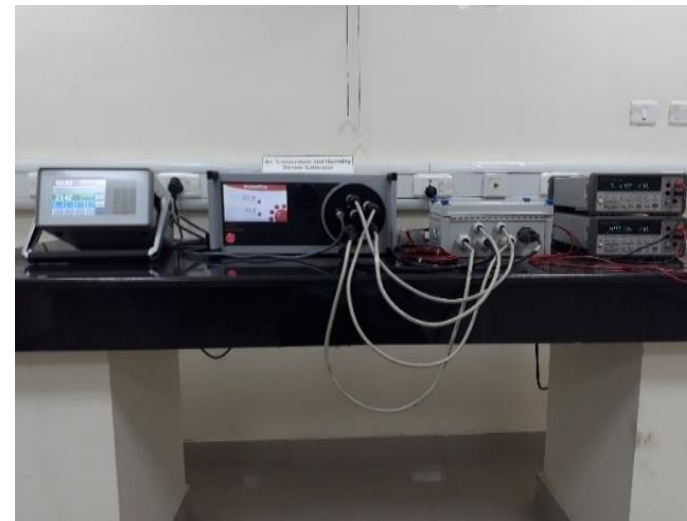
Chilled mirror and PRT Air temperature and Humidity sensor calibration
