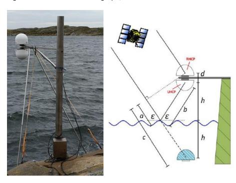
**Figure 11.** An upward- and downward looking GNSS-reflectometer.
