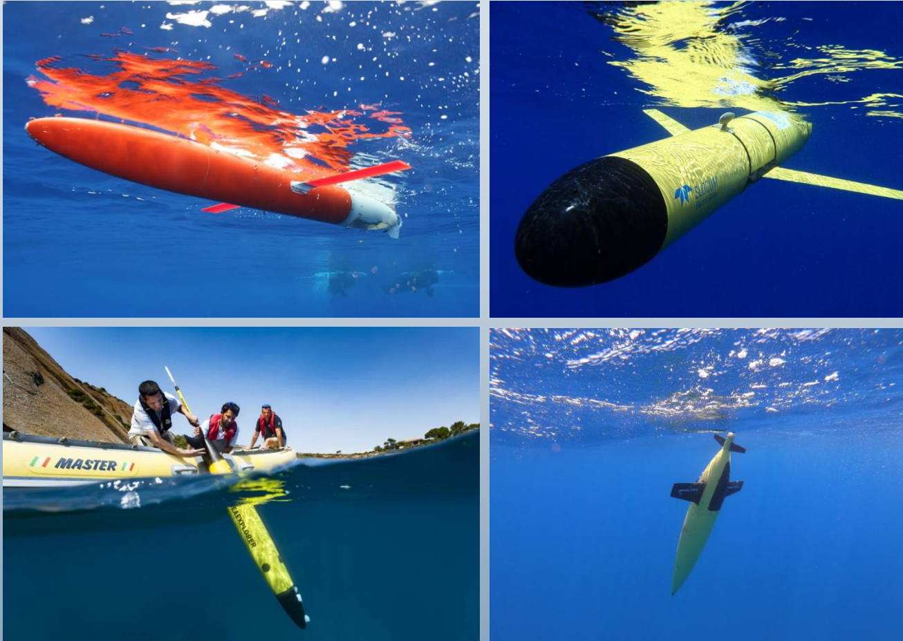
The different glider models. From top left to bottom right: Spray, Slocum, SeaExplorer, SeaGlider
