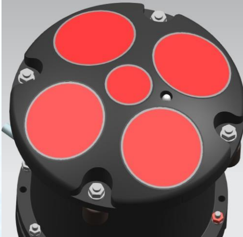
Transducer acoustic transmission layer
