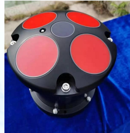
Transducer acoustic transmission layer
