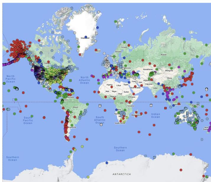
**Figure 2** Distribution of broad-band seismic stations sending real-time data to IRIS DMC. Figure 2 shows the uneven distribution of land-based seismic stations contributing open data to the global system. In addition, the monitoring system of the Comprehensive Nuclear-Test-Ban Treaty Organization (CTBTO), composed of 170 primary
