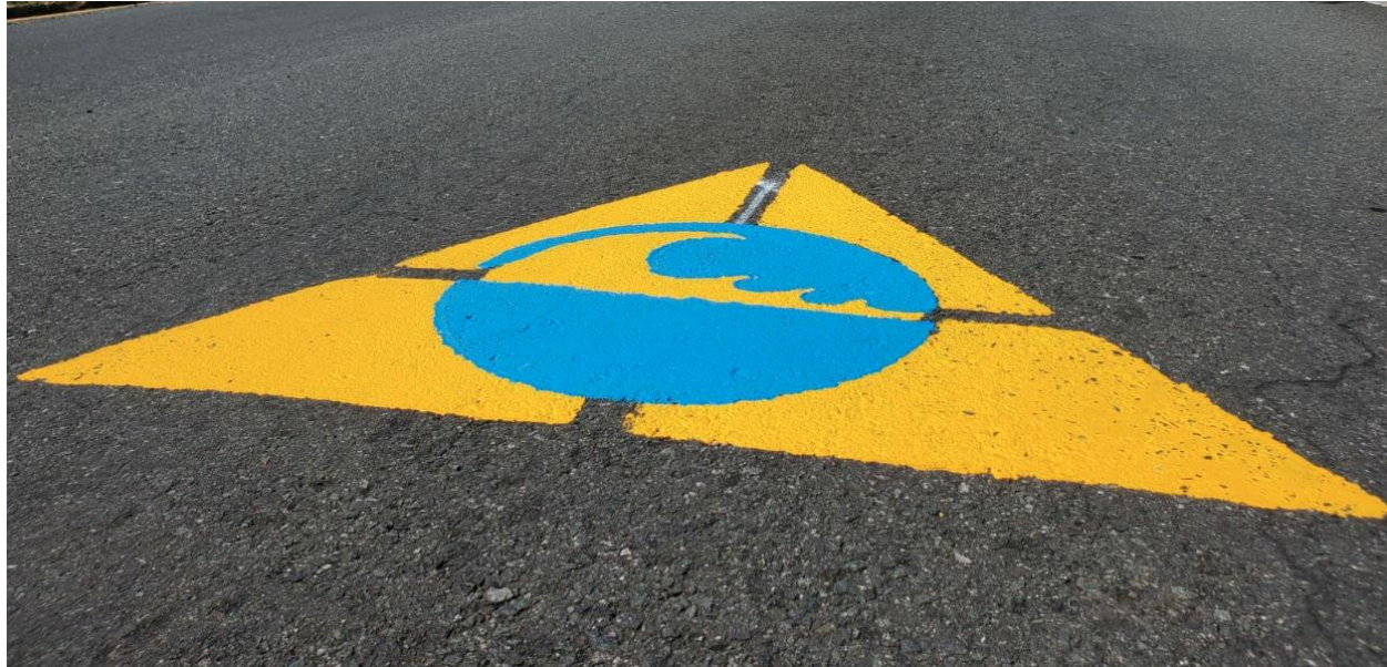
Figure 4. Tsunami evacuation route road marking in Toa Baja, Puerto Rico. More pictures online.
