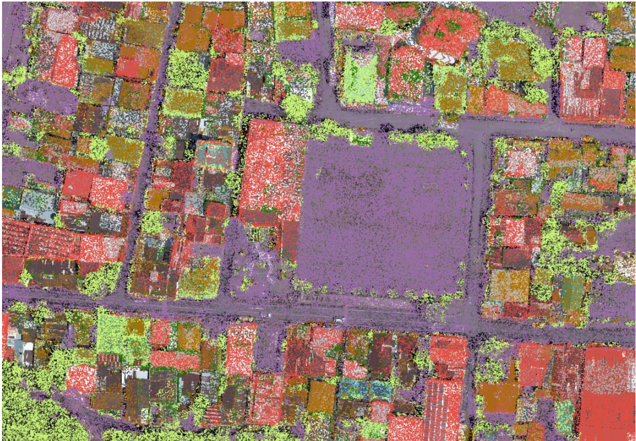
Illustration 7: Classified LIDAR point cloud. The purple and brown color indicate the natural terrain and roads. Red dots indicate buildings. Light and dark green colors indicate vegetation.
