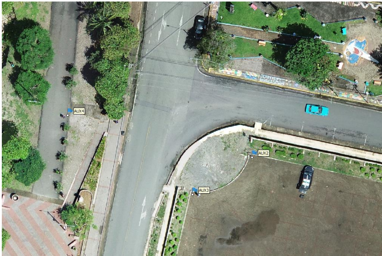
Illustration 3: Location of reference points for flight, generated from the MOPT reference points.
