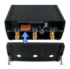
To insert the SIM in the router, remove the router from the control box with a small cross screwdriver (two small screws at the side of the router), and open the router as shown in the figure.
