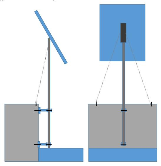
The figures below show the details of the connection of the wires at the bottom, with the tensor, and at the top, with the solar panel. To fix the wires we used nautical shackles, needed to prevent the corrosion from the sea water.
