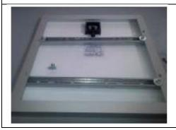
Repeat the same procedure with the other bar and keep a distance between the two bars approximately 50% of the length of the panel. Again, <u>do not</u> fix the bars strongly
