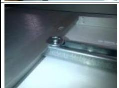
It is better  $\underline{\mathsf{not}}$  to fix completely the bar to have the possibility to a final adjustment
