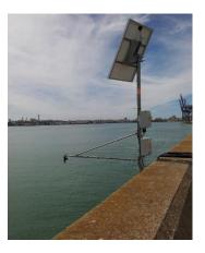
The horizontal angle should be towards south (0). The vertical orientation of the solar panel depends on the latitude of installation. The following table may serve as indication. The orientation can also be computed approximately as follows>
