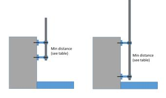
Once identified the right vertical wall that allows the fixing of the supports with their minimum distance, it is usually necessary to involve specialized personnel (Fire Fighters or Mountain specialists) that will work hanging outside the vertical wall to drill and fix the supports.
