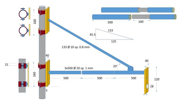
The sensor arm is composed of a number of stainless-steel pieces to form a triangular shape with a final part containing a hole in which the sensor is installed. The horizontal part can be at the bottom or at the top of the triangle depending on the local conditions.
