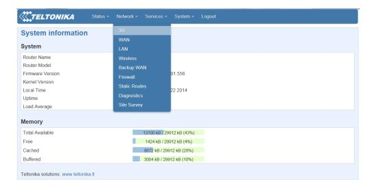
Change the APN according to the GSM provider (in the image below web.omnitel.it) and the PIN number of your SIM card, if any. The Dialing Number in general should be left blank or \*99# and the authentication mode as none. If your phone card provider require authentication, indicate CHAP or PAP from the drop down menu and a user/password fields will appear. For the service mode leave 3g preferred, if available in your area.
