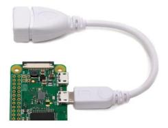
Connect the power charger (microusb) to the first port. The power supply should provide 1.2A (see Power Supply specs)
