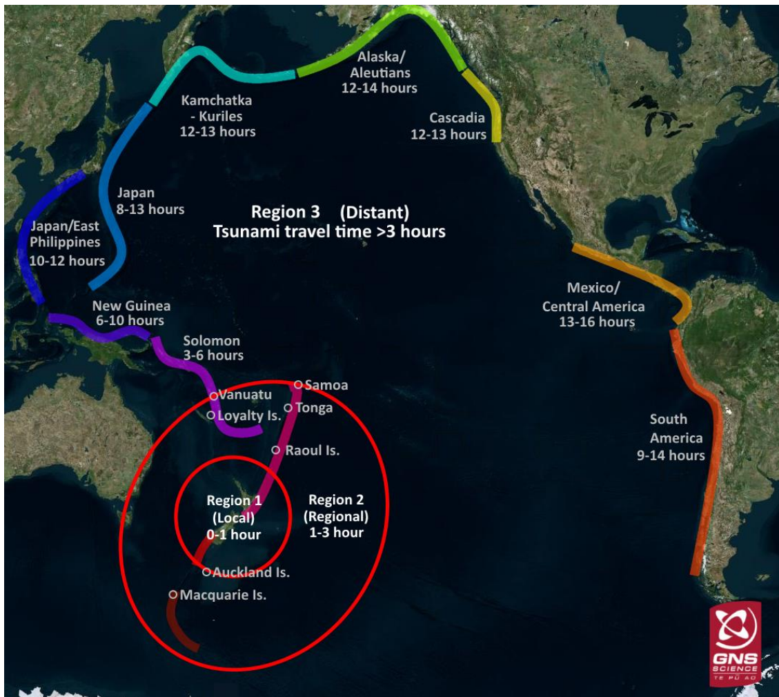
Figure 1: Local (1), regional (2) and distant (3) source regions based on minimal tsunami travel time to New Zealand shores
