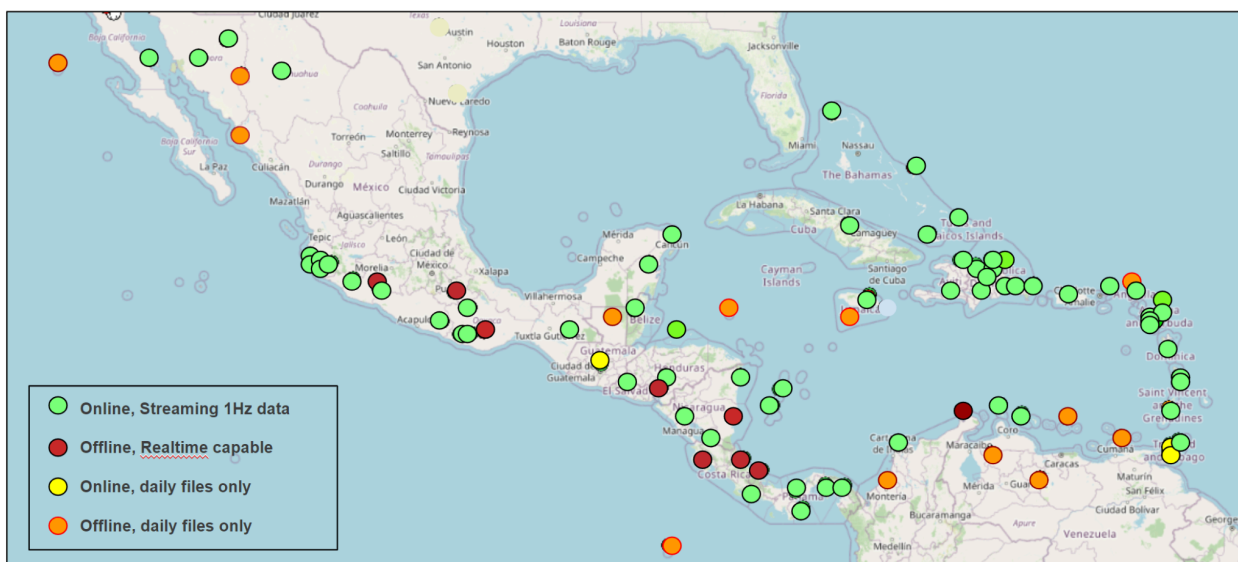
Figure 5. Caribbean regional GNSS assets within the Network of the Americas (NSF-GAGE Facility operated by the EarthScope Consortium). This includes 67 stations that are currently operational and streaming 1-Hz data which could be utilized for tsunami hazard monitoring.
