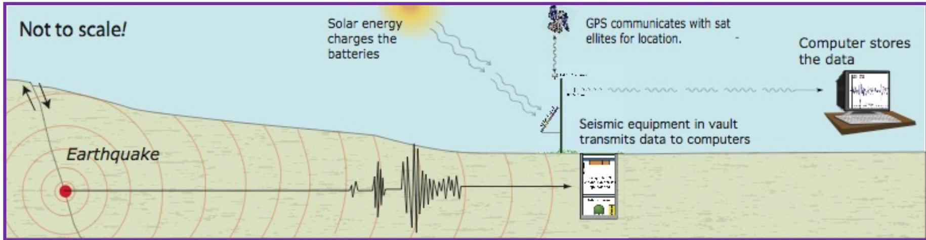
When an earthquake occurs, the seismic waves travel through the Earth to the seismic station where the information is transmitted to distant computers.
