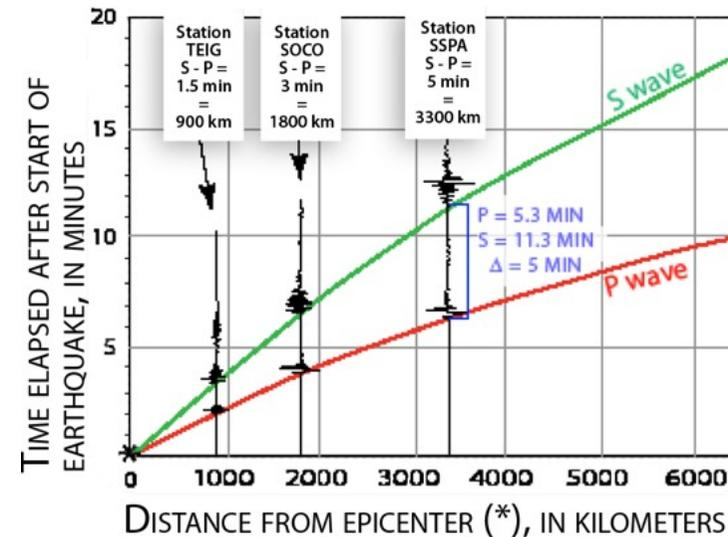
1. Determine distance of EQ from three seismic stations by calculating the S minus P arrival times.
