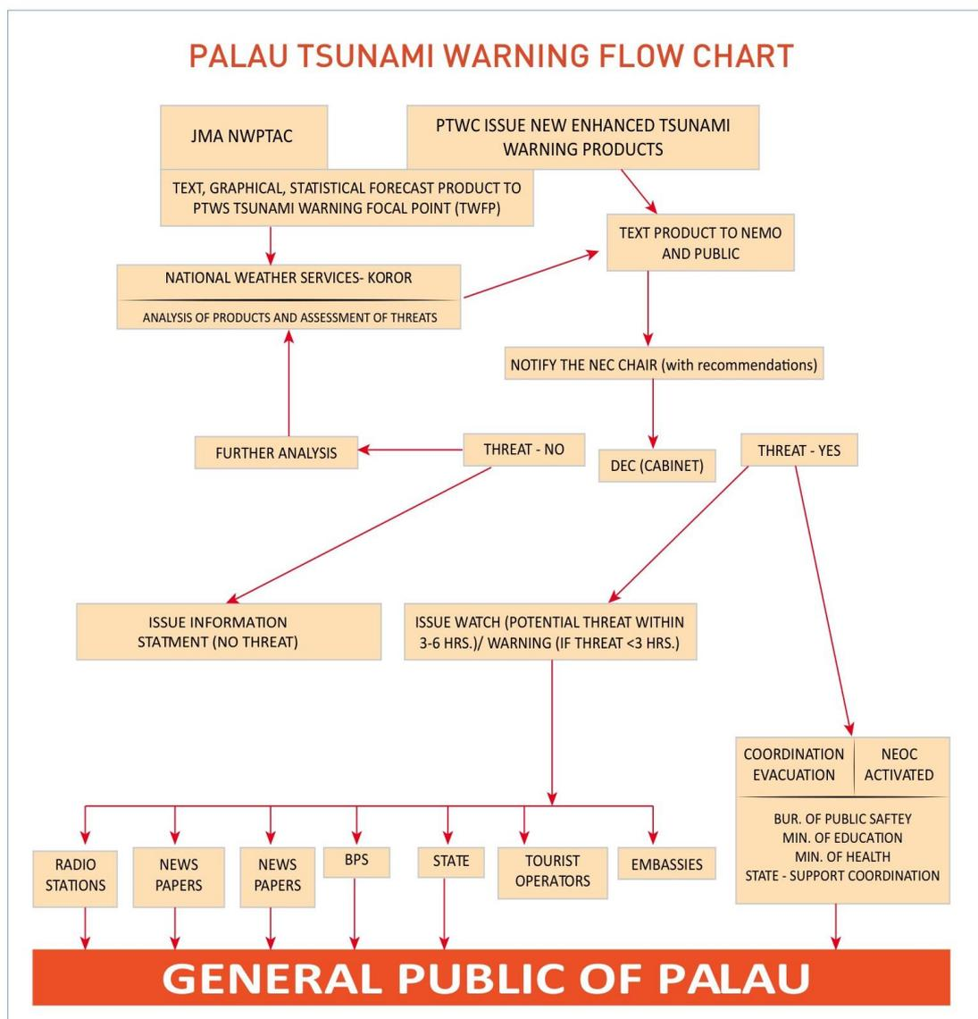
**Example of PTWC flow chart (2011) of procedures leading to issuance of its initial bulletin**
