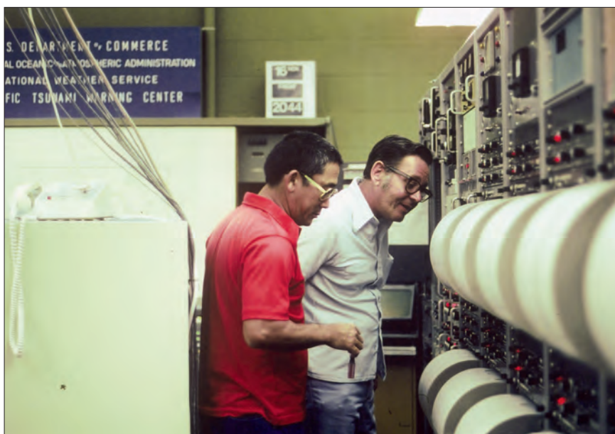
Heliocorders were used into the 1990s to monitor seismicity. Watchstanders measured P-wave arrival times and wave amplitudes off the rotating ink drums, and input their readings into a computer to calculate the hypocenter and surface wave magnitude. (Credit: ITIC archives)
