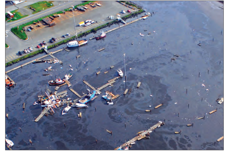
Crescent City, California boat harbor damage after the 2011 Japan tsunami. Strong wave currents entering the enclosed harbor (from top of photo) formed an eddy, which was left in the sediment swirls. The tsunami caused USD $55 million in damage to moorings and vessels in two dozen harbors in California. (Credit: R. Hiser and L. Dengler)
