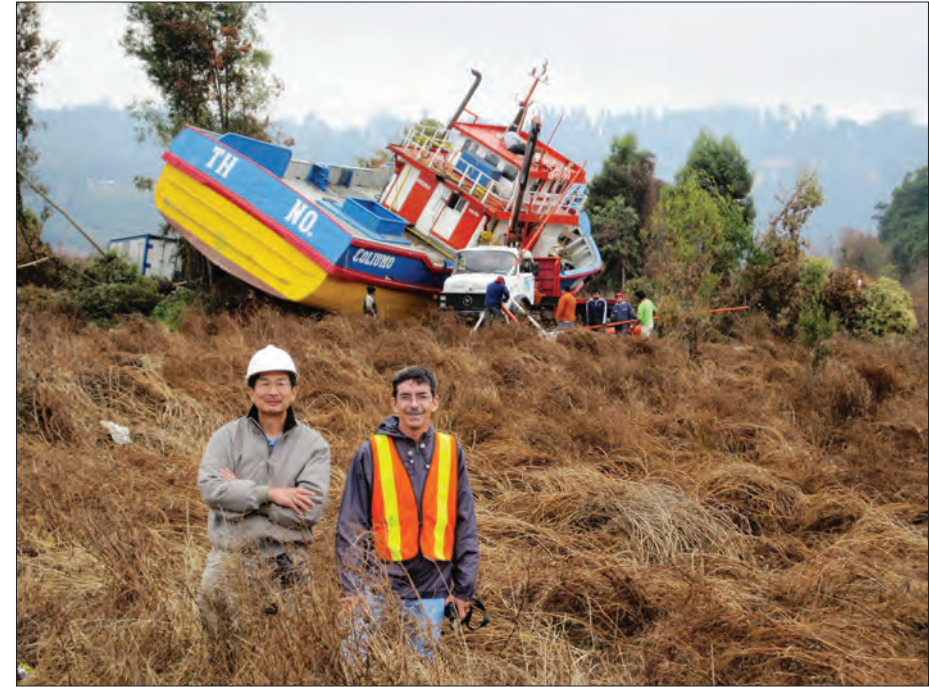
Fishing boat was carried inland several kilometers near Coliumo, southern Chile. Brown vegetation that died from sea water immersion delineates maximum tsunami runup. ITST-Chile post-earthquake and tsunami surveys by engineers documented structural impacts. (Credit: G. Chock, I. Robertson)
