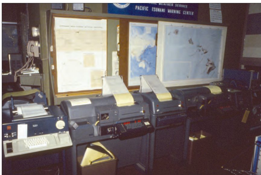
Tsunami messages were disseminated by teletype through the 1990s. Messages were punched onto paper tape and run through the encoder for transmission over the Defense Communication System that connected to the NOAA NWS gateway for distribution throughout the Pacific. (Credit: ITIC archives)
