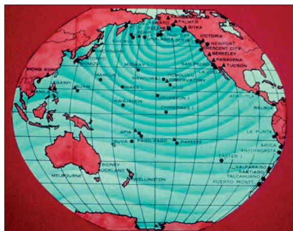
Seismic (triangle) and Sea Level (circles) reporting stations for the Tsunami Warning System in the Pacific. In early 1970s, there were 31 seismic stations, 48 tide stations, and 23 countries cooperating.
