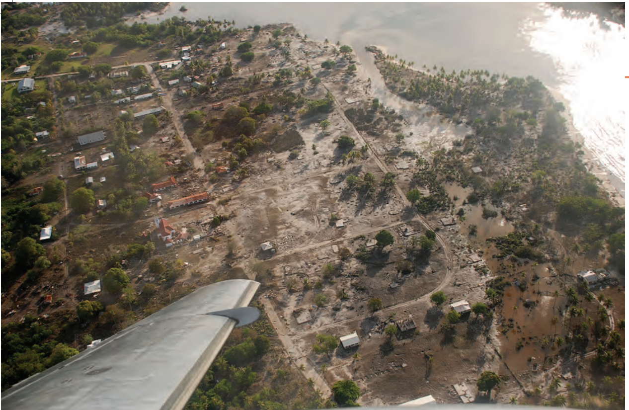
Figure 10. Hihifo, Niutopotapu, shattered by a tsunami. Concrete foundation slabs show where the business centre stood, while the remains of homes are scattered over the area. Aerial reconnaissance, 30 September 2009.
