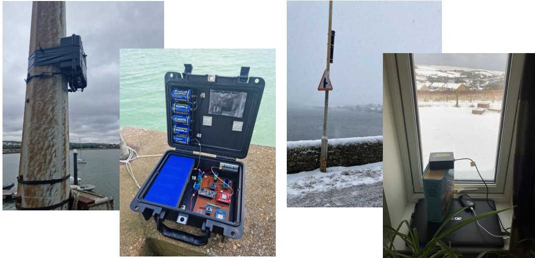
Figure 12. Some examples of low-cost GNSS-IR sensors
