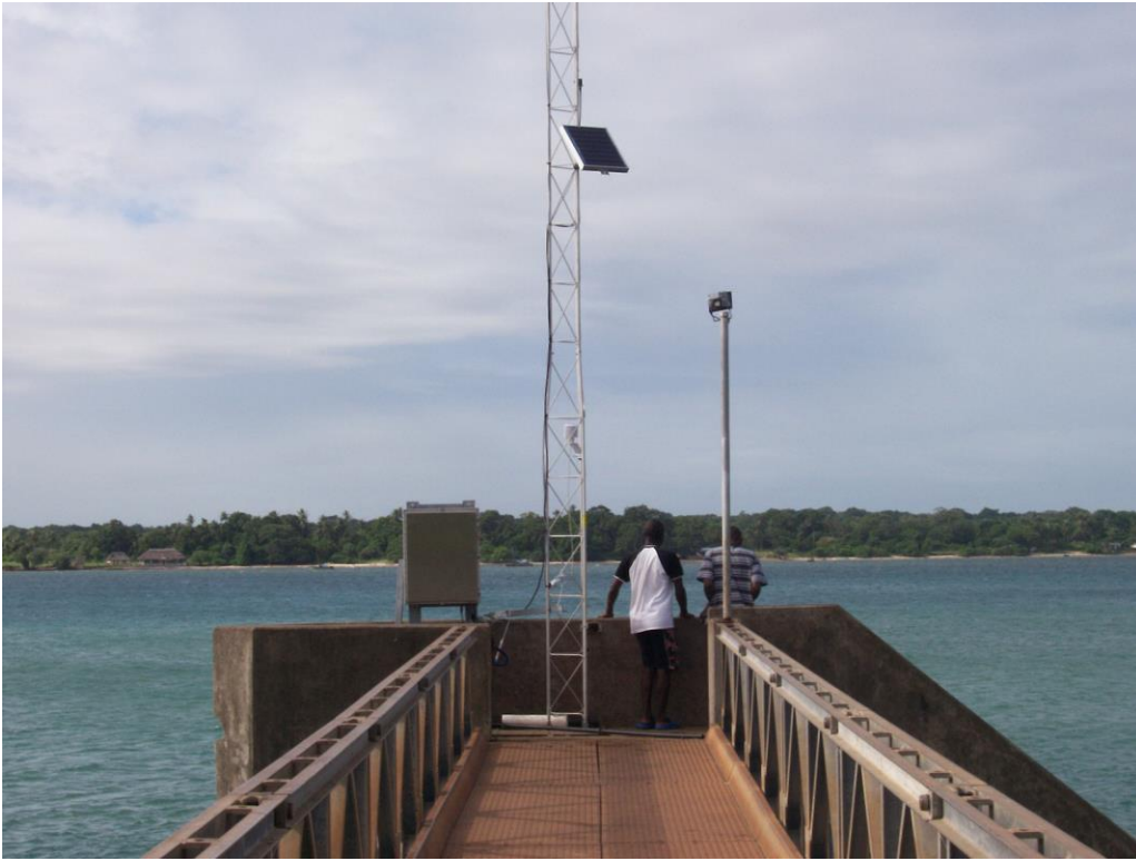
Fig5a: Wasini Island Tidal and Automatic Weather Station installed at the Old Navy Jetty
