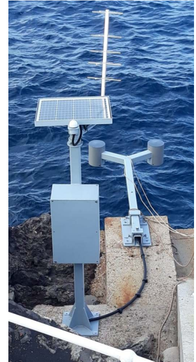
Renewable powered twin radar at Ascension
