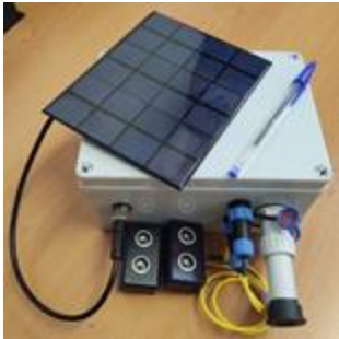
Low-cost Sea Level Sensor (in collaboration with Univ. Tuscia)
