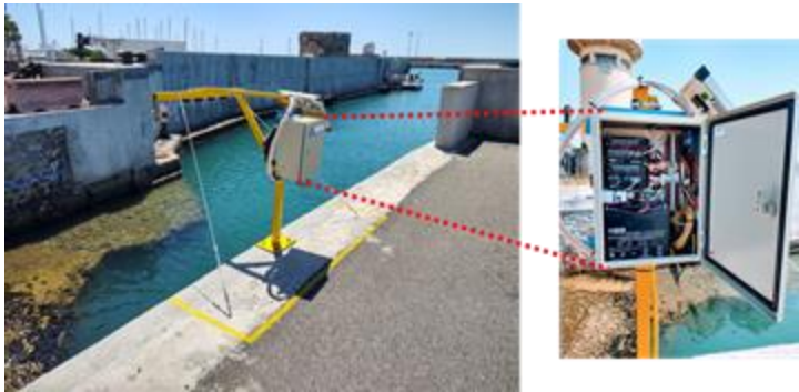
Low-cost Sea Level Sensor (in collaboration with Univ. Tuscia)
