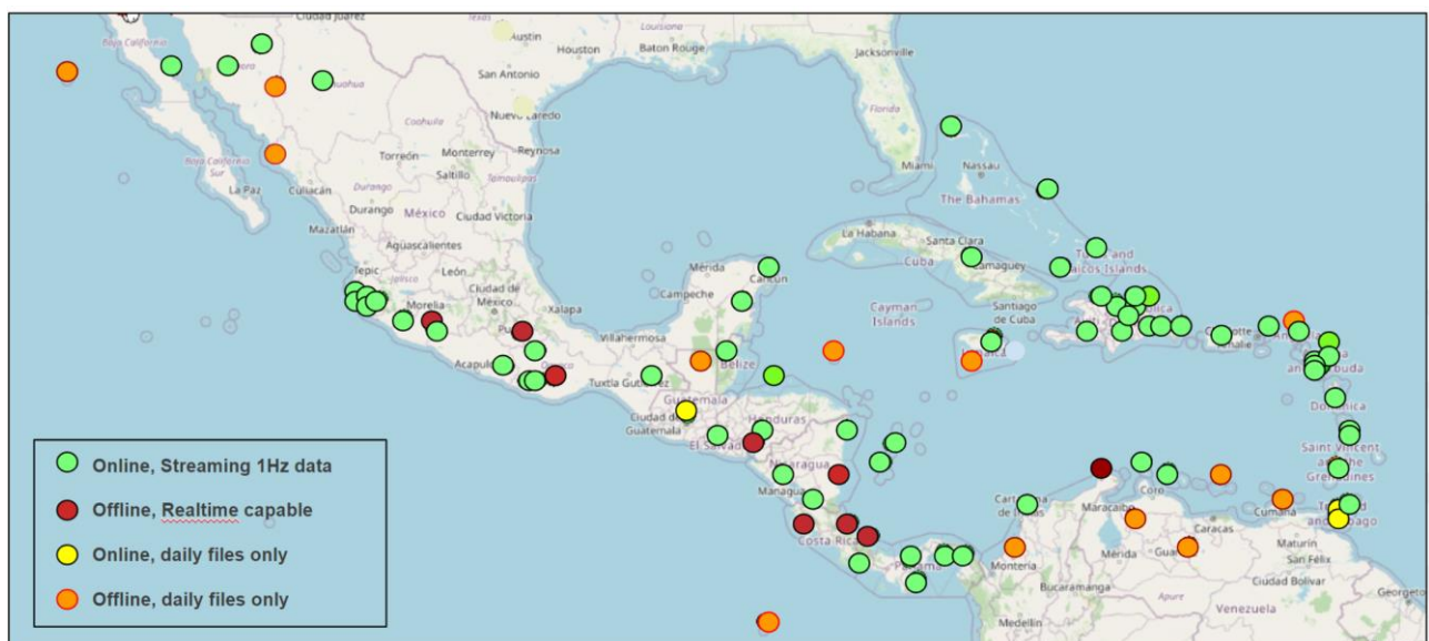
Figure 8. Caribbean regional GNSS assets within the Network of the Americas (NSF-GAGE Facility operated by the EarthScope Consortium). This includes 67 stations that are currently operational and streaming 1-Hz data which could be utilized for tsunami hazard monitoring.
