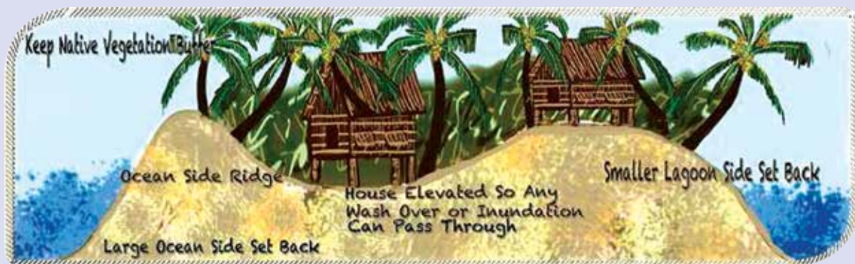
Figure 4-55. From the UH Sea Grant publication “A Landowners Guide to Coastal Protection.” The ocean side of the atoll receives more wave energy and consists of courser grained and steeper ridges or berms. The lagoon side has smaller ridges and finer sediment. It is important to build and maintain migratory and fixed ridges or berms. Also re-vegetate the shoreline below the high water mark with mangroves and above with other suitable salt-resistant varieties.
