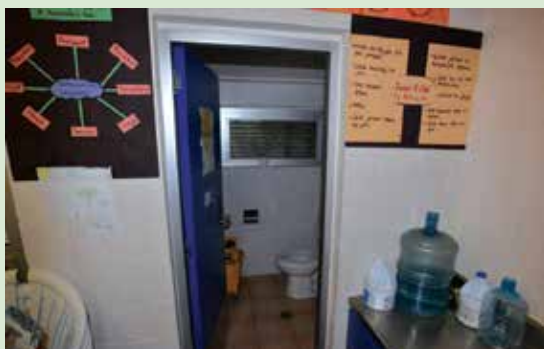
Figure 3-15. An ideal shelter will have toilet facilities available on the same floor as the shelter. This is common in newer elementary schools. Other comfort criteria include minimum space standards such as 10 square feet per person. In an emergency, these criteria may be compromised in the interests of accommodating more people in the shelters.
