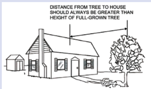
Figure 4-49. FEMA recommends keeping trees a distance greater than the height of a full grown tree. This will prevent roof damage from strong winds and also reduce risk that leaves will fall on your roof and enter the water catchment system.
