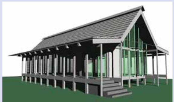
Figure 4-48. This experimental, affordable house is designed to withstand typhoon and storm surge events. Elevation would be from 4 to 8 feet off the ground on reinforced concrete piers similar to those in Figure 4-40, 4-41 and 4-45. Once the pier foundation is set, wall frames are erected using stainless steel connection plates. Strong prefabricated panels are then used for the floor, walls and roof. The panels are made of cement, fly ash, sand and polyvinyl alcohol fibers to give it added strength (From Rockwood, et al, 2015 in Prep.).
