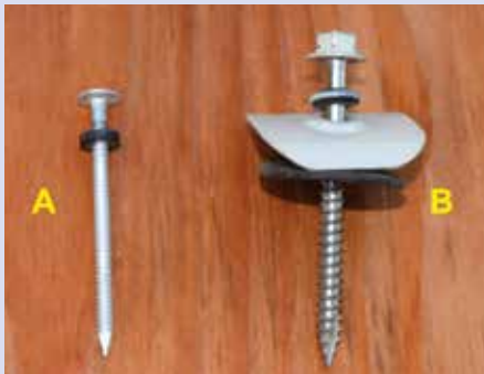
Figure 4-21. Different fasteners to tie the metal corrugated roof to the Purlins. (A) Aluminum ring shank nails with rubber washer is a strong method to attach the aluminum roof. Material is readily available in Majuro. (B) Aluminum screw with rubber washer, aluminum metal cap and another rubber washer is an even stronger method to tie the metal roof to the purlins. Unit cost is about $1. The Majuro Department of Public Works ordered these in bulk to attach the roofs for the local schools.
