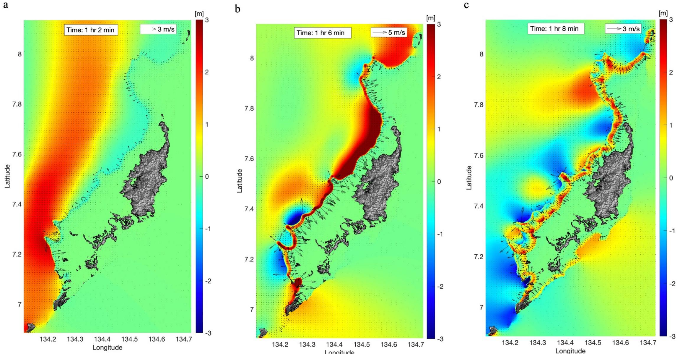
The wave amplitudes (offshore) and tsunami heights (onshore) and currents (black vectors) at different time intervals after earthquake from the Philippine2 source, the most dangerous for Koror.
