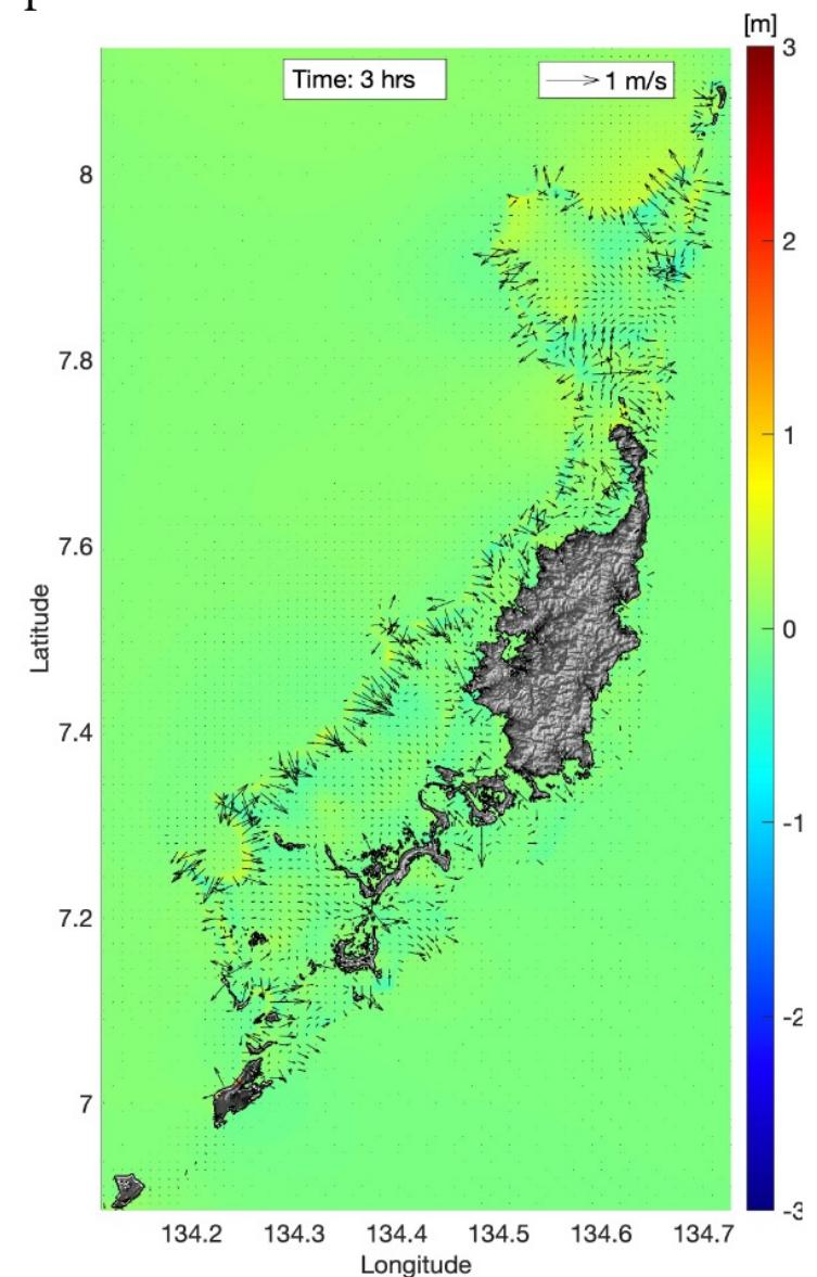
The wave amplitudes (offshore) and tsunami heights (onshore) and currents (black vectors) at different time intervals after earthquake from the Philippine2 source, the most dangerous for Koror.
