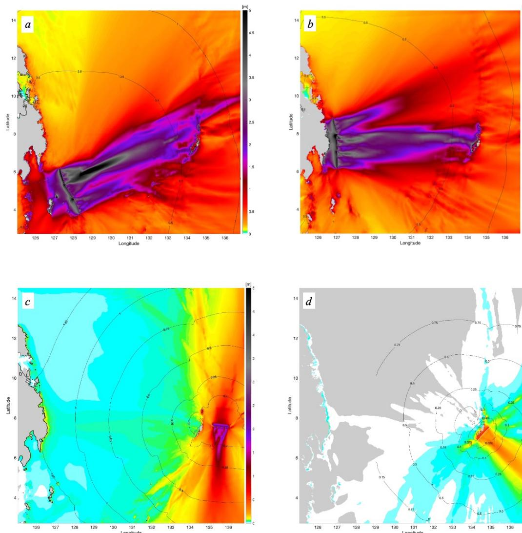
Source location, arrival times, and maximum wave amplitudes in deep ocean for the most hazardous sources Phillipine1 (a), Phillipine2 (b) and the closest to Palau significant impact sources Yap (c) and Palau (d).
