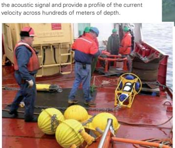
Preparing for deployment of a mooring with hardhats, an ADCP, acoustic releases and the bottom anchor. (Fiamma Straneo, Woods Hole Oceanographic Institution)
