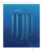
The direct sampling of ocean water by lowering bottles from a ship and returning water samples shipboard for analysis remains one of the fundamental tools of ocean observations. The workhorse of hydrography is the Niskin bottle which is often deployed
