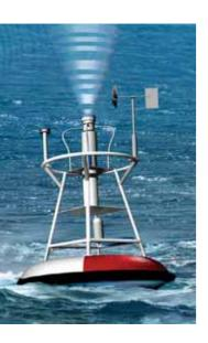
information collected by a network of DART® systems currently positioned at strategic locations in the Pacific. northwest Atlantic, and eastern Indian Oceans plays a critical role in tsunami forecasting. The first information available about the source of a tsunami comes from seismic monitors tracking disturbances along the seafloor. If the landslide or tectonic event is large enough to generate a tsunami wave, the DART® buoys, recording sea level measurements.
