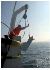
The CPR is about one meter in length. The body is made of gunmetal, (phosphor bronze), or stainless steel in later versions from 1997. The CPR has been operated successfully at speeds of up to 25 knots, and its robust design allows deployment in rough seas without fear of excessive damage. Successful tows
