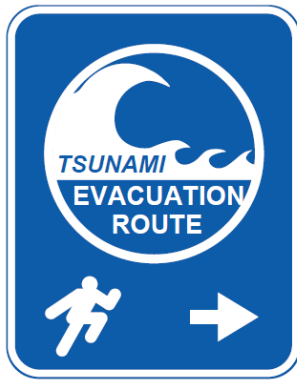
Figure S.46. Tsunami evacuation walking sign
