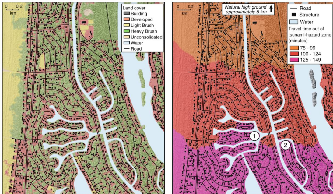
Figure S.53. Maps showing modelling inputs (left) and calculated 'least-cost', pedestrian-evacuation travel times (based on a travel speed of 1.1 m/s, right) for the central portion of the incorporated city of Ocean Shores, Washington (Wood and Schmidtlein, 2013a). 'Least-cost' refers to the calculation of the 'cost' (in terms of travel time) due to the varying landscape (roads, landcover, elevation, buildings, etc.),
